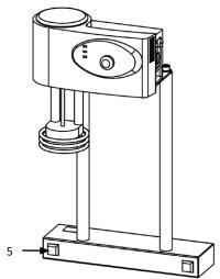
The 1 litre measuring cylinders must be placed in the glass tank (use the weighting ring for a stable set-up). The glass tank is filled with water of a temperature that is kept at as constant a level as possible with the aid of the heating element with thermostat and stirring element (art. nr: 083010).
