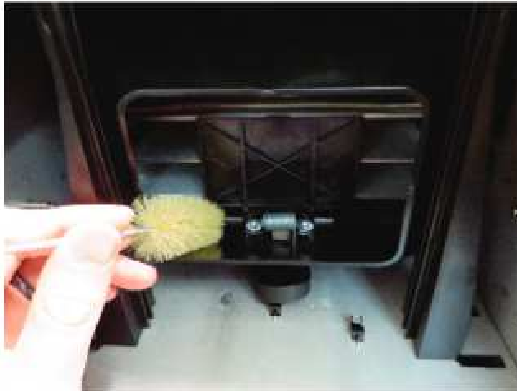
Figure 12 Clean Under Trap Door
