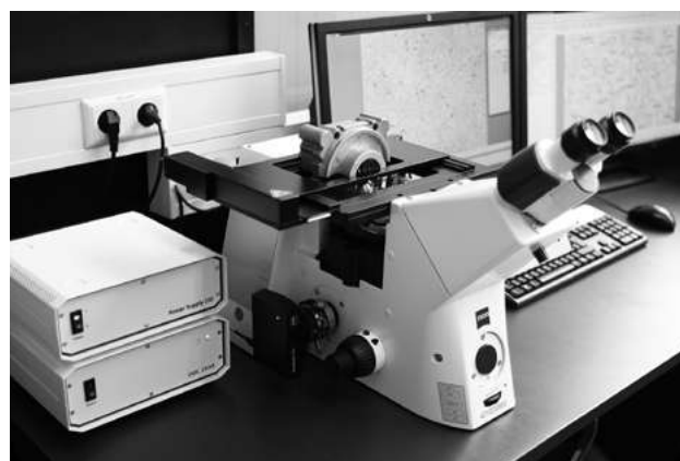
Figure 1 Microstructural analysis of macrosections of larger nonferrous cast components. The inverted design of the microscope makes it easier and quicker for users to conduct their analysis. Samples do not need to be sectioned and mounted; those being inspected are positioned directly at focus level, allowing even large and heavy samples to be examined directly.
