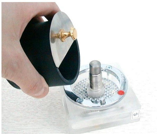
Figure 15: Fill in the sample into the bottom part of the measuring cell
