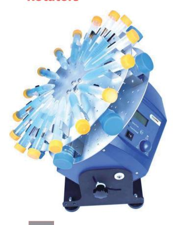
SCILOGEX rotators give gentle but effective mixing of biological samples held in 1.5mL to 50mL tubes, and are used in a variety of applications including immune precipitations, prevention of blood coagulation, latex diagnostics, etc.
