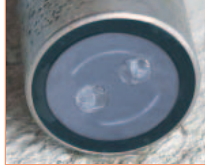
Sensor with ultrasound cleaning system After 16 Days
