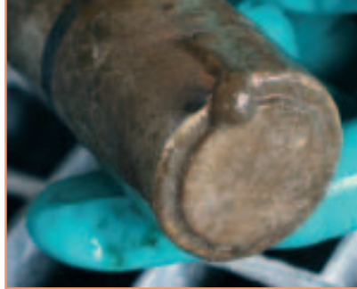
Sensor without ultrasound cleaning system After 16 Days
