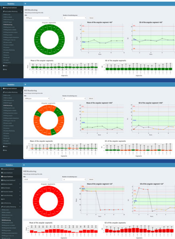
Dashboard in PrepMaster Analytics for the Tool Condition Monitoring Module for vibratory disk mills
