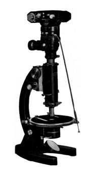
Shutter speed: B, 1—1/250sec. Size of image: 24mm X 36mm Specimen can be photographed during observation Has insertion opening for photo cell of photomicrographic exposure meter. Has smooth, stable shutter performance. Magnification on the film plane is about 1/3x of microscope total magnifications
