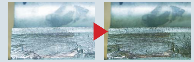
Four-part illumination of surface fracture (metal)
