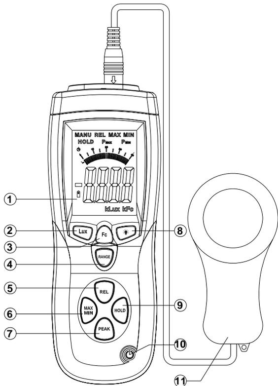
1. LCD Display: 3-3/4 digit displays with a maximum reading of 3999, and the indicating signs of measured values, unit function symbols and decimal points etc are display.
