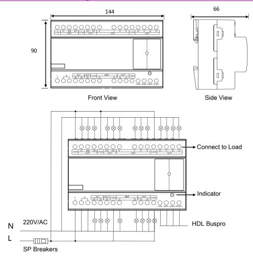
**Indicator:** flickers when the module is working properly. Keep pressing for 3 seconds, it can be read and modify the start address in the HDL-Hotel Room Intelligent System Manage Software.
