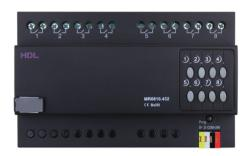
HDL-MR0810.432 Intelligent Relay Module, has 16A launching relay inside, Zero power consumption and high reliability. The relay's communication interface is HDL Bus Pro, which is based on RS485 protocol.
