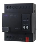
HDL-M/DALI.1 HDL KNX DALI module can connect up to 64 DALI devices for address assignment and management.it can be real-time to detect the device fault, such as DALI fault,Lamp fault,Ballast fault. For each channel and group, supports Switch ON/OFF , Relative dimming , Absolute dimming,1bit and 1byte statues response function. Supports the KNX standard dimming curve and DALI standard dimming curve.
