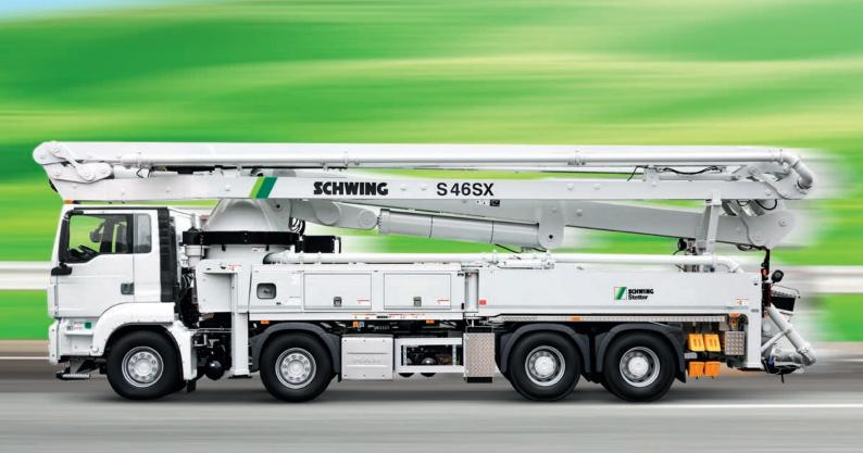
Vertical reach 45.6 m Concrete output max. 162 m³/h Pressure on concrete max. 85 bar
