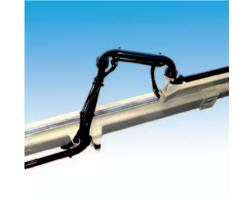
The RZ boom can be telescoped by 4,60m during a pour without increasing the resistance of the concrete flow in the pipe line.
