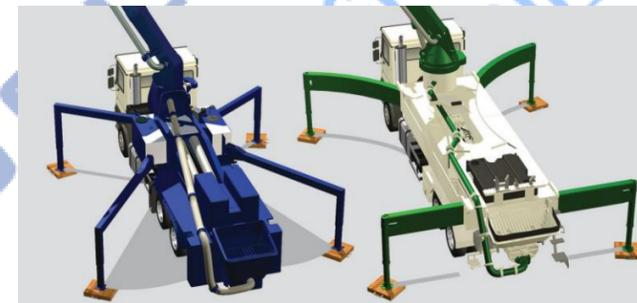
Due to the combination of front X and rear H outriggers the S 34 X can set up without the space hogging footprints of the other outrigging systems.
