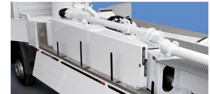
The torsion resistant frame that transfers the outrigger forces directly to the corner points provides enough space for a 600l oil tank and room for hoses and pipes.
