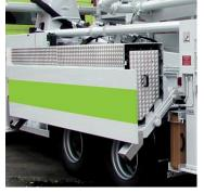
In the hydraulically lowerable boxes the hoses are comfortably accessible at operator height.
