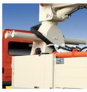
Two slewing cylinders on each side assure safe operation and longevity of the turret.
