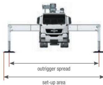
The outrigger spreads as specified are measured from the centre of the outrigger leg. Any cribbing or underlay timbers must be taken into account when determining the required set-up area.
