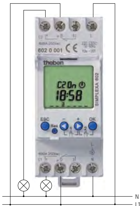
SIMPLEXA 602 – Connection diagram
