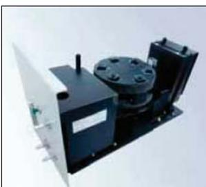
Constant temperature 6 place cell changer, 10mm cuvettes, ideal for Kinetics.
