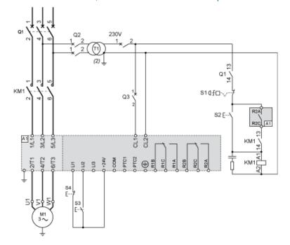
With Line Contactor, Freewheel or Controlled Stop
