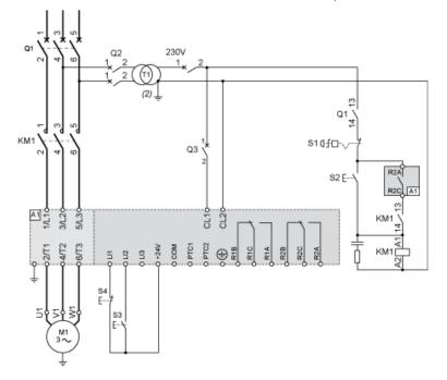
With Line Contactor, Freewheel or Controlled Stop
