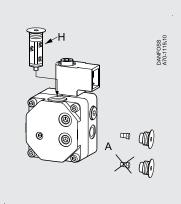
2-pipe operation: screw fitted
