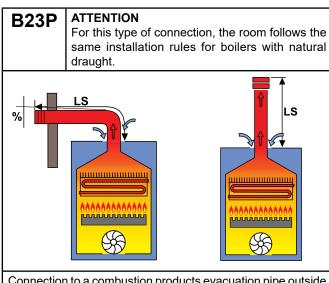
Connection to a combustion products evacuation pipe outside the room; the combustion air is taken directly from the room where the appliance is installed.
