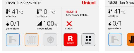
Fault that causes the boiler to stop:
