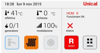
Fault that does NOT cause the boiler to stop: - The error code is displayed, the boiler has a heating request, Reset icon (informing that a failure has been detected, even if the fault was temporary). Therefore, you must always carry out reset to cancel the word "Error" displayed.
