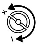
(S) ADJUSTMENT SCREW MAXIMUM OUTPUT (R) ADJUSTMENT SCREW MINIMUM OUTPUT
