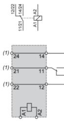
(1) Terminals 11 and 21,14 and 24,12 and 22 must be linked for this references **NOTE:** For DC input, A1 have to be +, otherwise it would short circuit from protection module
