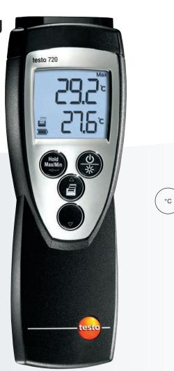
The testo 720 is a robust temperature measuring instrument for precise air, surface and immersion measurements in the measuring range from -100 to +800 °C. It is possible to connect Pt100 probes as well as NTC probes to the onechannel measuring instrument.
