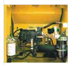
The engine oil filter, the large fuel filter (with built-in water separator) and the additional large water separator are remote mounted and easy to reach from ground level. Both the fuel filter and the water separator, which remove contaminants and water, have an important function forengine performance and durability.
