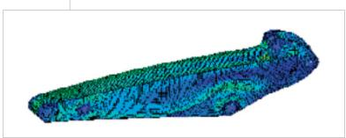
Booms and Arms have been redesigned using advanced CAD (Computer Aided Design) and FEM (Finite Elements Methodology) Systems to get higher strength **only** in those areas where stresses are concentrated.
