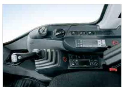
All switches and controls are now positioned at the right side, easy to find and to reach. The radio and the new, more effective automatic air-conditioning system are standard equipment, creating an agreeable working atmosphere regardless of the external weather conditions. The joystick illustrated is supplied as an option, together with rotating bucket circuit.
