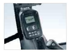
The newly designed **A.E.P. Information Display** features analogical gauges which provide one sight advice, regardless of the operating environment. The digital display screen has been enlarged to further enhance visibility.
