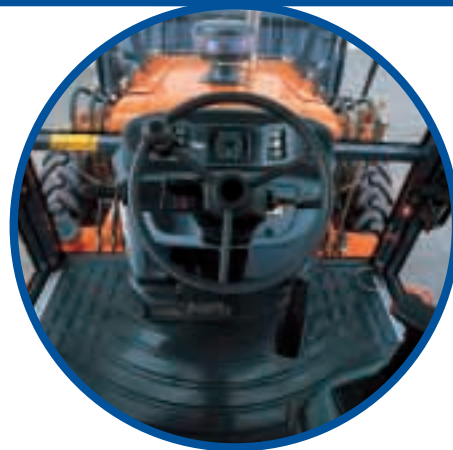
Excellent positioning of the transmission control lever Foot pedal operated accelerator and brake pedals, for easier operation.
