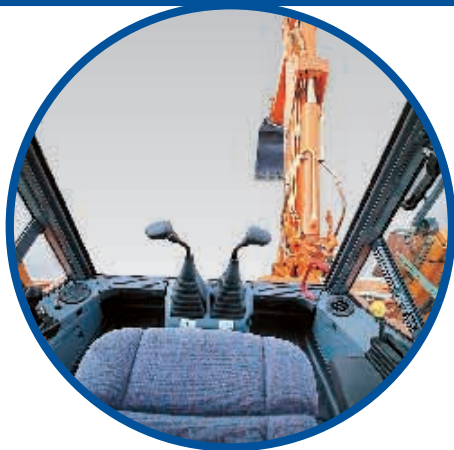
Backhoe controls Standard controls are mechanical Soft and precise backhoe controls are positioned ergonomically to offer maximum operator comfort and all-round visibility of the digging area.
