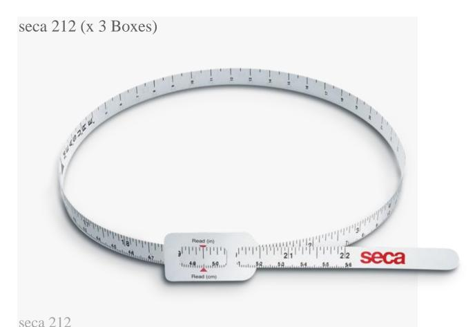
A scale on each side permits measuring of head circumference and facial symmetry.
