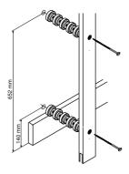
You select the distance of the measuring rod to the wall with the number of spacers on the screws. You must use at least one washer for each of the two fixing points.
