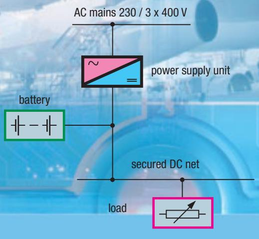
Fig. 2: Standby parallel operation
