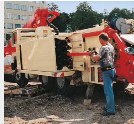
The container can be lowered hydraulically to make handling the pipes and hoses simpler (option, only available in conjunction with a 4200 mm wheelbase)
