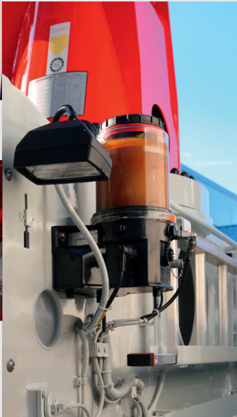
The central grease lubrication system on the boom reduces the time for daily maintenance
