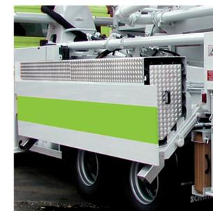
In the hydraulically lowerable boxes the hoses are comfortably accessible at operator height.
