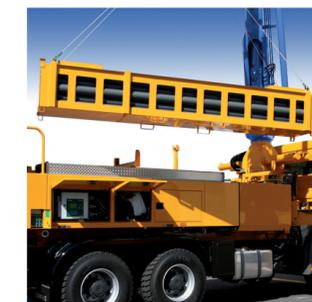
The hose storage boxes on the right side can be loaded and unloaded by a fork lift, crane or the pumps own boom.
